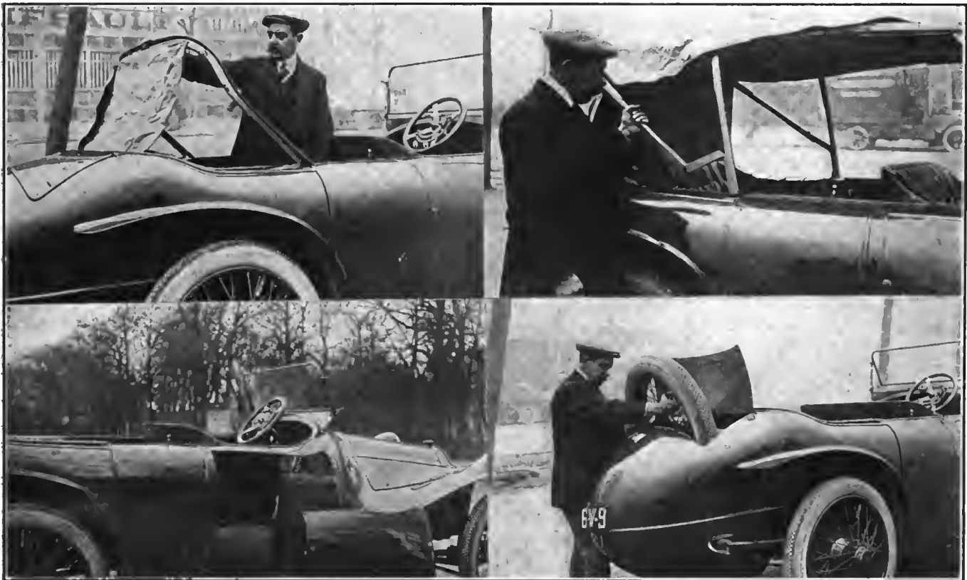
Showing the way the top folds into the body on the Turcat-Mery torpedo and baggage and spare wheel compartments
